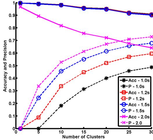
Fig. 6: Plot illustrating the trade-off between accuracy and precision as the number of clusters increase, when  $T = 1.0, 1.2, 1.5,$  and  $2.0s$ .
