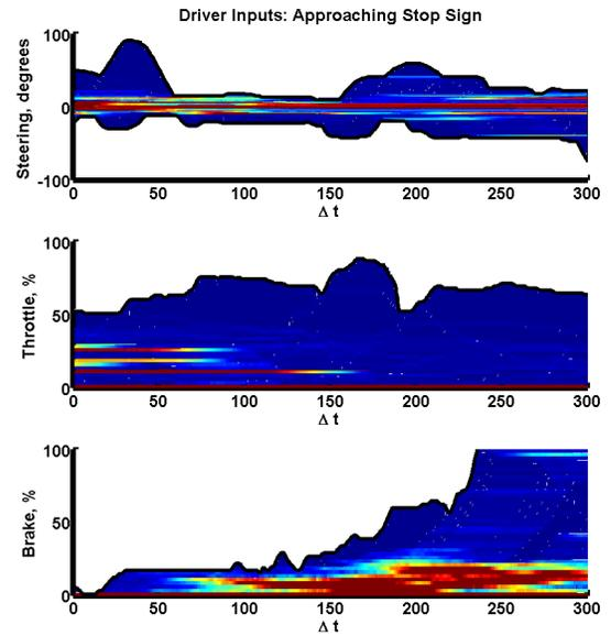
Fig. 10: An example set of driver's inputs when approaching a stop sign, associated with the trajectory set in Fig. 9a.
