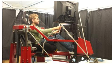
Fig. 3: Picture of test subject driving the simulator.
