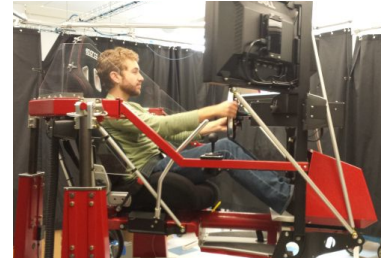
Fig. 4: (Left) The validation study asked the driver to indicate when the autonomous vehicle (shown in red) was about to change lanes from view 1, as a passenger in the driver seat, and from view 2, as another vehicle on the road. (Right) Motion simulator originally used to collect the dataset, and used to validate the different control schemes.
